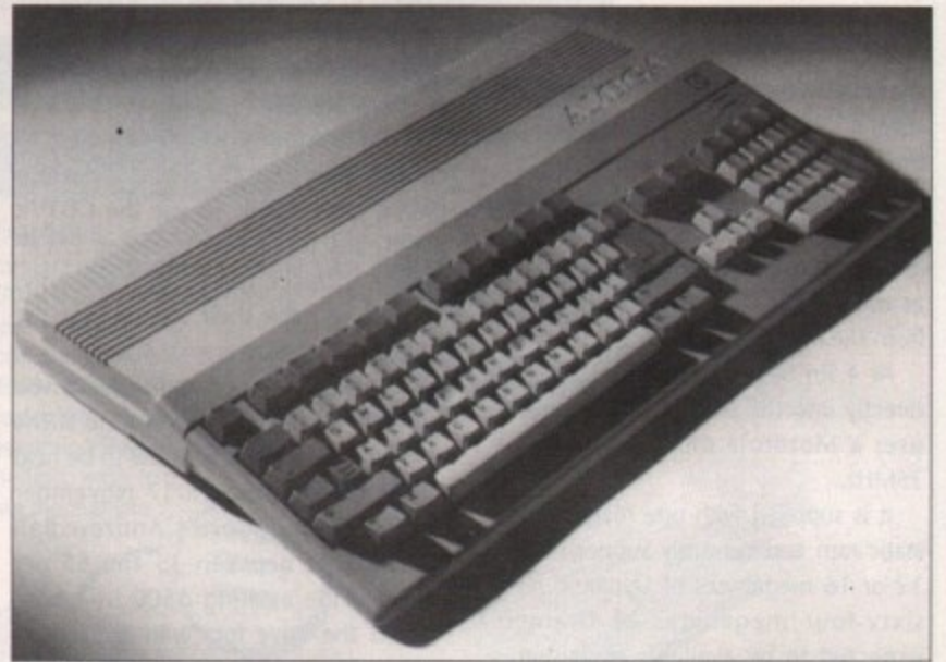
On the outside the A500P looks identical to the A500, but inside there's a full megabyte of memory, the enhanced chip set and an improved operating system
